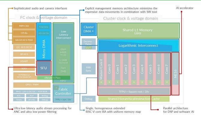
GAP9 is a unique combination of a powerful low power microcontroller, a programmable compute cluster with a hardware neural network accelerator and sample by sample audio filtering unit.
